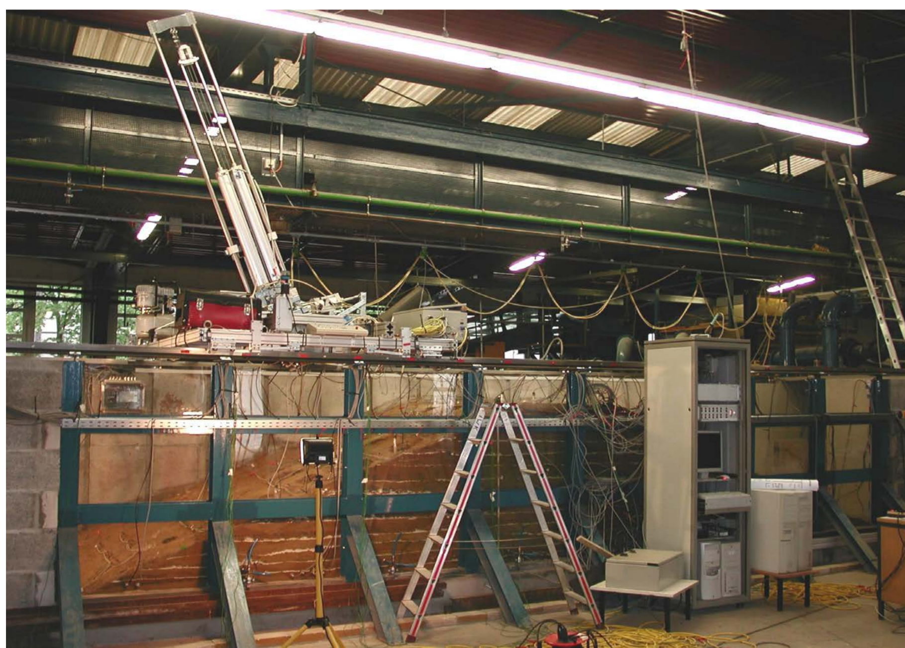
Fig. 2: Test facility at the Theodor-Rehbock-Laboratory, with model dikes according to a proportion of 1:3 to 1:4 of real dikes
