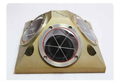
Laser reflectors developed at the GFZ are mounted on the satellites. They reflect laser light emitted by selected observation stations (including stations at the GFZ). From these measurements, the distance to Earth and thus the orbit can be determined very precisely.
