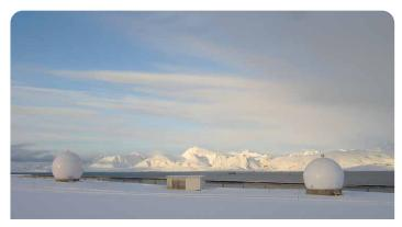
GFZ's own receiving station on Spitsbergen is located near the North Pole allowing for contact with the satellites almost every orbit for timely provision of the data to the users.
