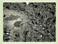
Reflected light image of an uranium-rich Alum Shale sample.
