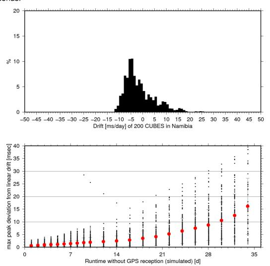
Remark: Please note the the CUBE was not designed to operate without GPS reception for a long time, GPS reception is considered as an integral part of the CUBE operation!
